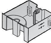
A 3D-style line drawing of a rectangular water tank. Inside, a coiled grey tube representing the intake hose is shown extending from the bottom left towards the center. The tube is depicted as being straight and vertical, representing the correct orientation for proper suction. |
