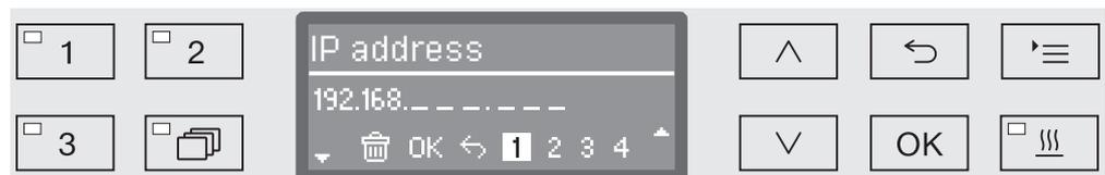
The current setting is shown on the middle line of the display. It can be changed using the options shown in the bottom line. The top line shows which option has been selected from the bottom line. The following data entry options are available:
