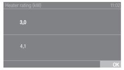
208 V  $\rightarrow$  3.0 kW heater rating 240 V  $\rightarrow$  4.1 kW heater rating
